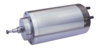
This product uses P4 grade high speed and high precision angular contact bearing and its cooling type is water cooled. The cooling water should be provided with sufficient flow, the pressure should be kept above 6 metres, and the cooling area of the cooling water tank should be large enough. The compressed air used shall be treated by dust removal and moisture removal. And the compressed air shall be with pressure of about 0.05Mp.
